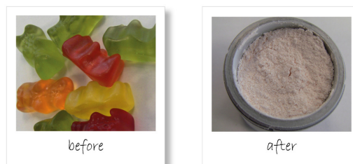
Fig. 8: Jelly bears before (left) and after cryogenic grinding in the Mixer Mill MM 400
