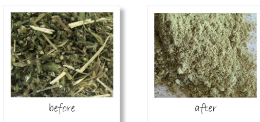
Fig. 4: After pre-cutting in the SM 400 XL (left) the sample is pulverized to <0.5 mm in the ZM 300
