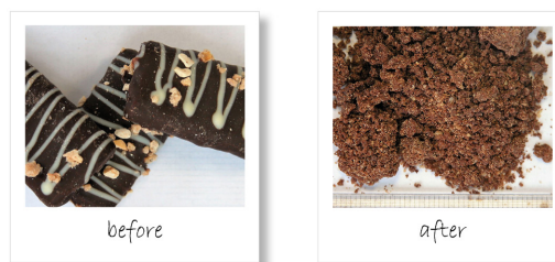
Fig. 10: Cookies before (left) and after pulverization in the Knife Mill GM 200 (right)
