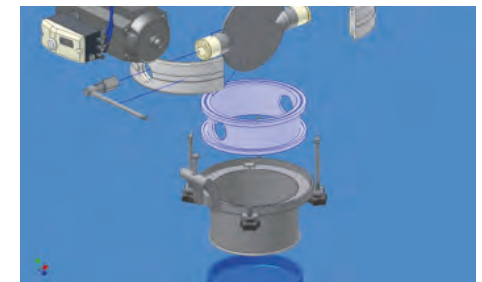
J-Tec quickly detachable dosing valve with dosing and sealing function
